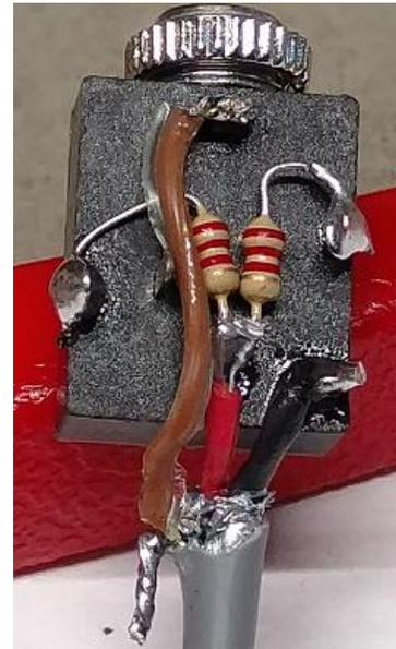
Here is the connection of the resistors and cable to the headphone jack.
