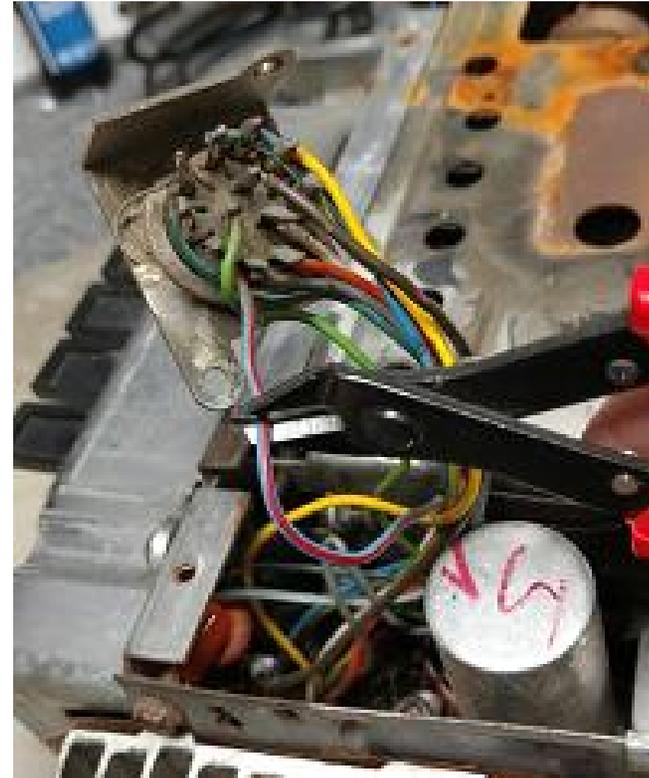
Lift out the socket to gain access to the wires.
