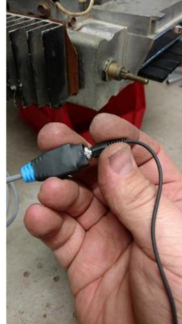
Connect the radio to power, speaker and antenna. With nothing installed to the AUX jack (Left Picture) turn the radio on. Radio should play a radio station. Verify the volume control adjusts the sound up and down.
